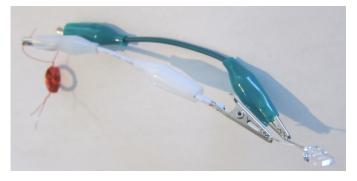
We will measure if any voltage is generated. The coil sees magnetic fields that come and go, generating **alternating current**. The meter does not have a sensitive AC setting, so we use the LED as a diode, to convert AC to DC, and set the meter to the most sensitive DC setting.
