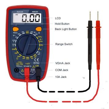
The **BLACK** lead plugs into COM (for 'common' or ground)
